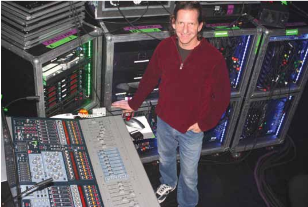
Doug Kimball's monitor beach with dual Venue Stage Racks and Sennheiser 2000 Series IEM transmitters. Below: Background singer and guitarist Marc Von Em's Digidesign PQ Controller and pick tray.
